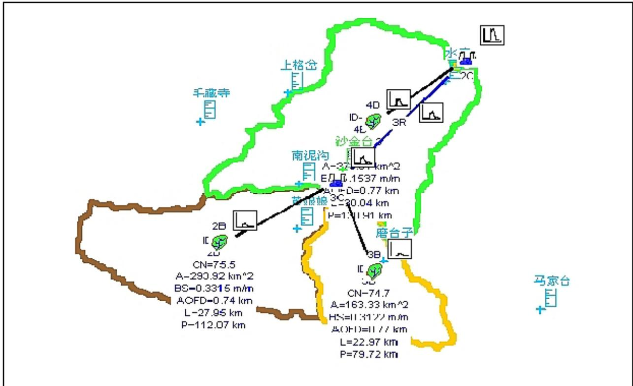
Figure 5. Topologic tree, gages, basin parameters and results.
