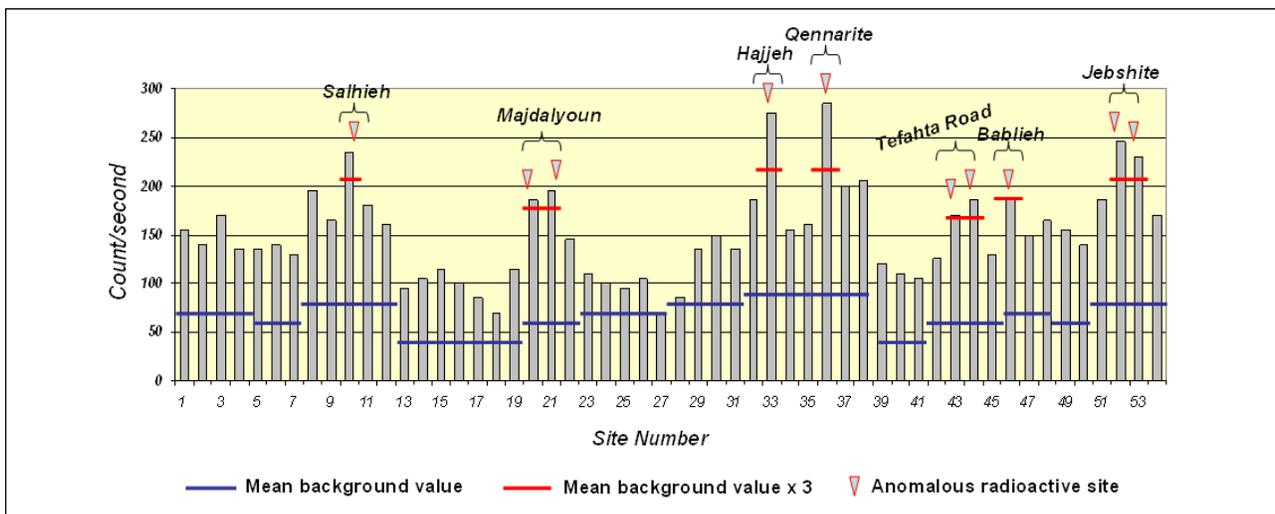
Figure 5. Graphic presentation of the radiometric survey in Saida-Zahrani and Nabatieh, showing the anomalous radioactive sites.
