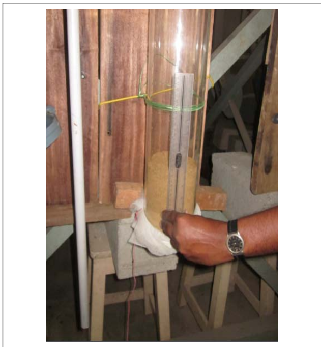
Figure 2. Soil packing in the columns.
