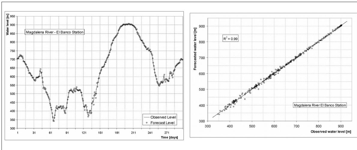
Figure 10. Comparison of forecast and observed water level (Equation 13) for the El Banco station with lead time  $T = 1$ .
