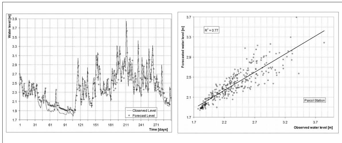
Figure 9. Comparison of forecast and observed water levels (Equation 12) for the Paicol station with lead time  $T = 1$  and using PERSIANN satellite-based precipitation estimates as exogenous predictors.
