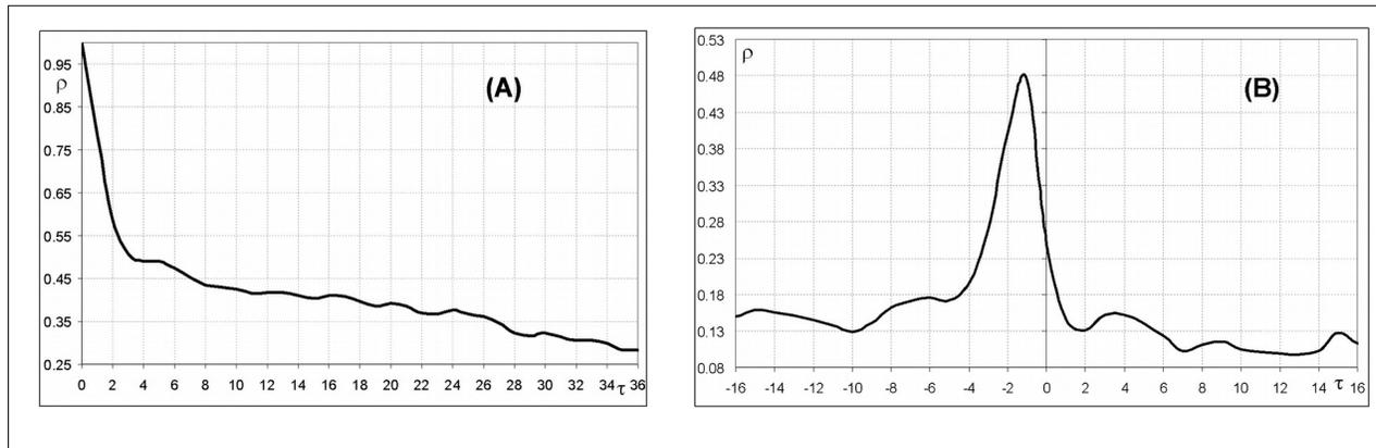
Figure 2. Streamflow autocorrelation (A) and rainfall/runoff cross-correlation (B) functions
