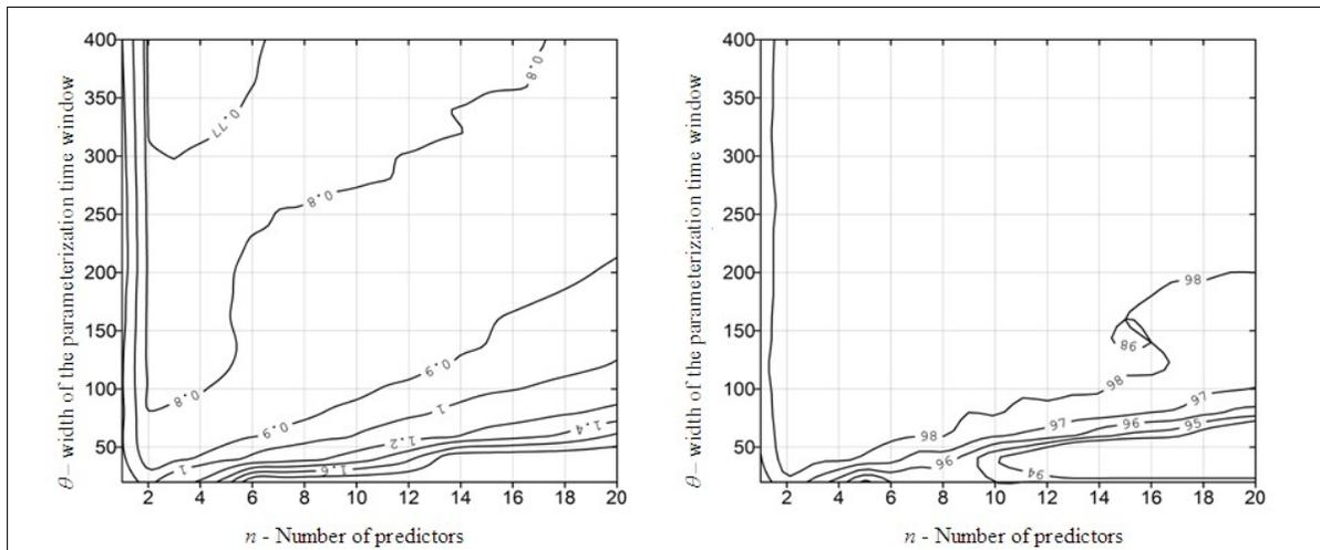
Figure 7.  $S/\sigma_\Delta$  behavior (left) and percentage of forecasts with error level  $\leq 5\%$  (right) using equation (22) to forecast El Banco daily water levels with  $T = 1$ .
