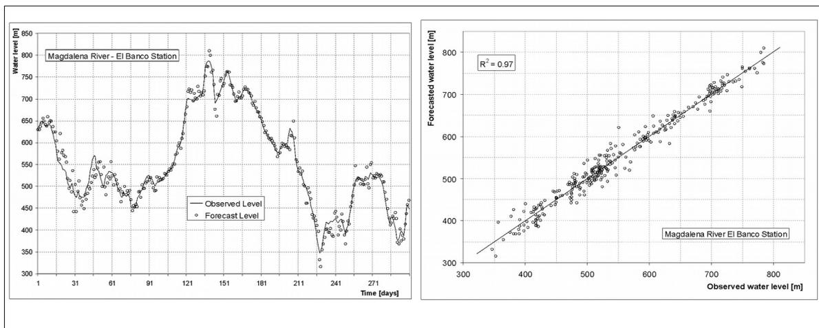
Figure 11. Comparison of forecast and observed water level (Equation 13) for the El Banco station with lead time  $T = 14$ .
