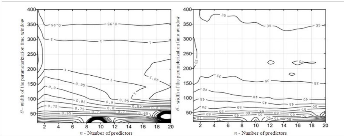
Figure 8.  $S/\sigma_{\Delta}$  behavior (left) and percentage of forecasts with error level  $\leq 5\%$  (right) using equation (23) to forecast El Banco daily water levels with  $T = 14$
