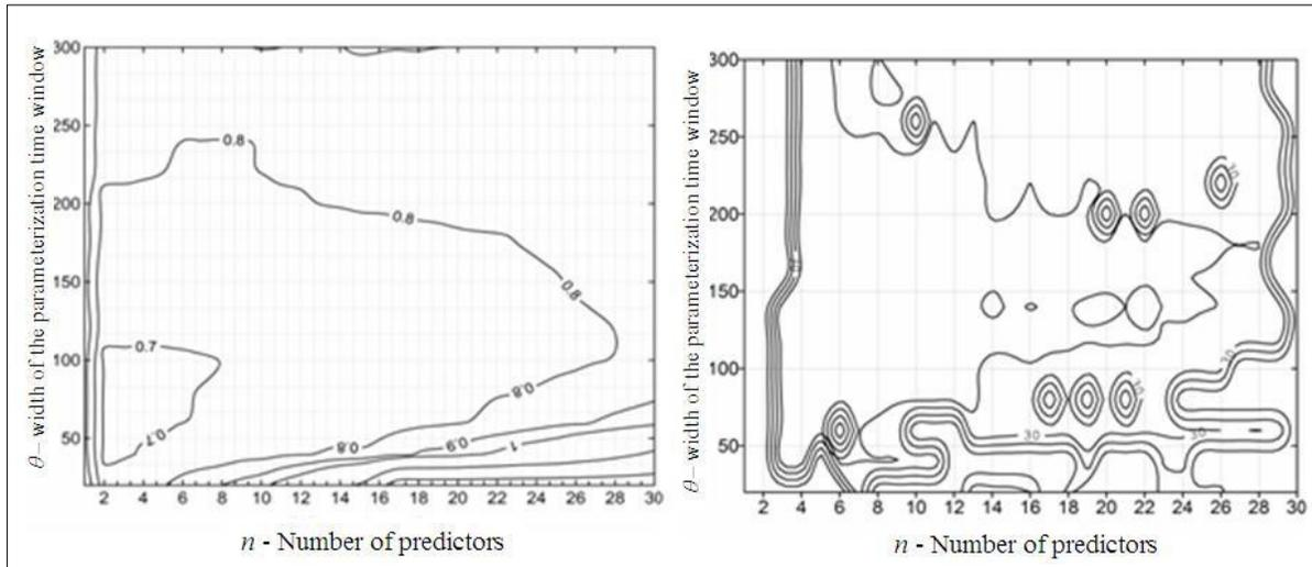
Figure 4.  $S/\sigma_{\Delta}$  behavior (left) and percentage of forecasts with error level  $\leq 5\%$  (right) using equation (19) to forecast Betania reservoir daily streamflows.
