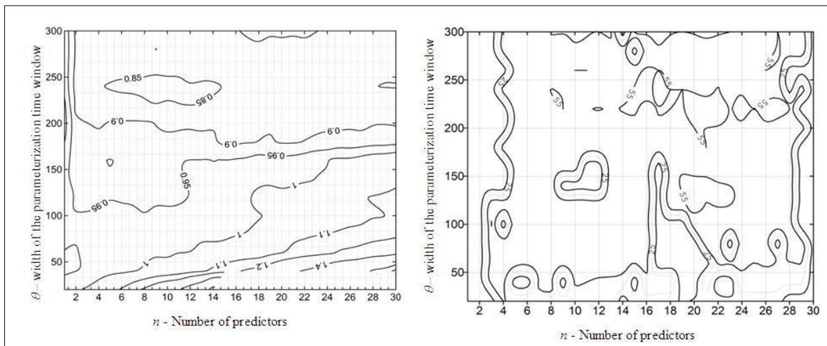
Figure 6.  $S/\sigma_{\Delta}$  behavior (left) and percentage of forecasts with error level  $\leq 5\%$  (right) using equation (20) and PERSIANN-based rainfall estimates to forecast daily stages at Paicol station
